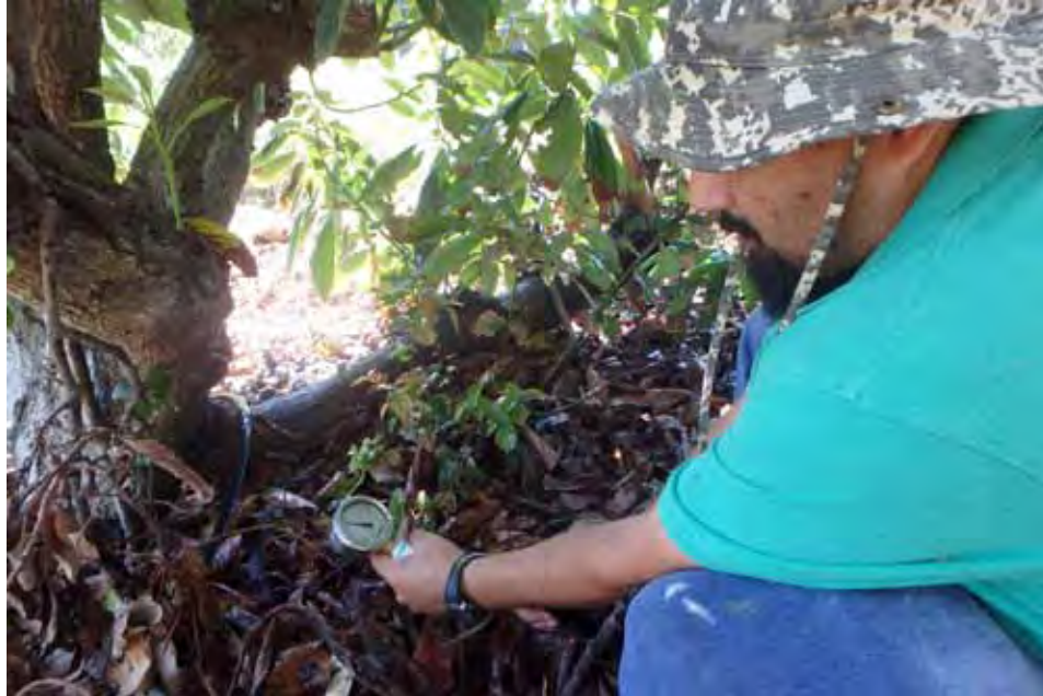
Jose Iniguez, irrigation auditor, tested water pressure to evaluate a sprinkler system for uniform distribution of water
